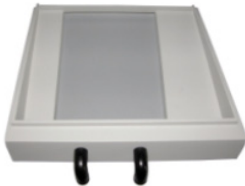
Fig. 10 SPEKOL® 1500 extension of sample compartment
