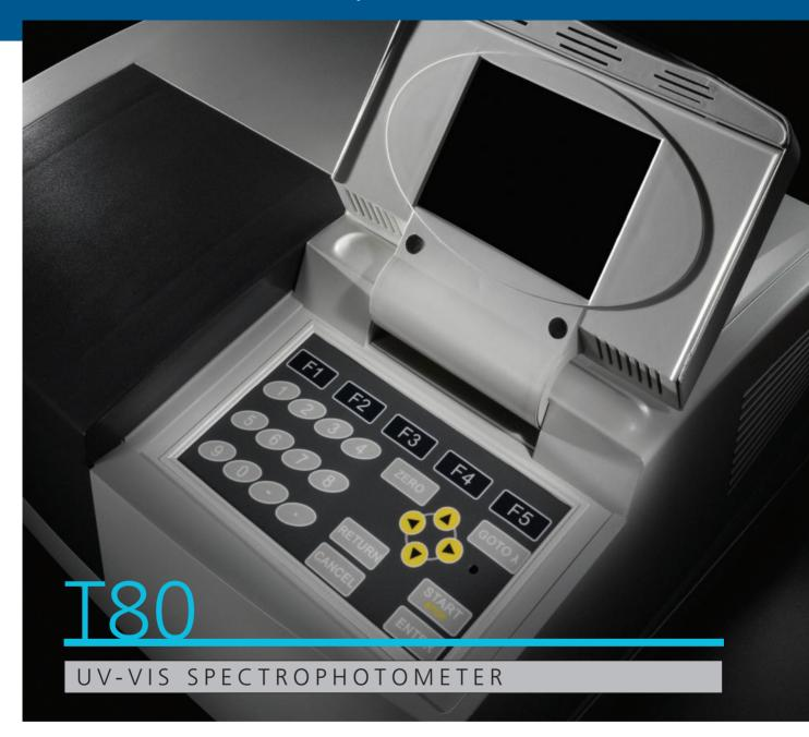
The T80 is a high performance double beam spectrophotometer available with a fixed (2nm) or variable (0.5, 1, 2, 5nm) spectral bandwidth, which is innovative in terms of instrument application, mechanical and optical design, electronic control and software whilst retaining features that are well established and accepted through the industry.
