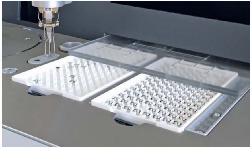
Two interchangeable pan trays plus one fixed strip yield a total of 204 positions for sample and reference pans; these are displayed here with the tray cover partially opened. Each tray can carry sample and reference pans of different types.
