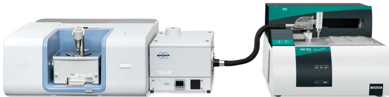
DSC 204 F1 Phoenix ® with ASC, coupled to the Bruker FT-IR spectrometer
