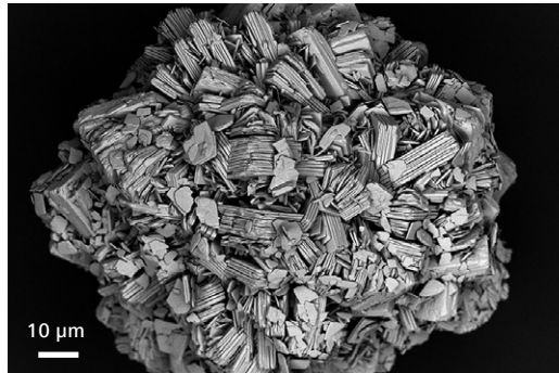
Lanthanum carbonate imaged at 1 kV with InLens Duo BSE. \text{LaCO}_3 is a phosphate binder used as a oral therapeutic agent for dialysis patients.
