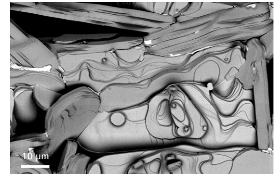
Super alloy sample imaged at 1 kV with the aBSD.
